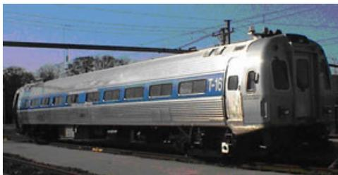
The ATIP program uses specialized vehicles that survey railroad tracks across the U.S. to identify track defects and exceptions. FRA works with the railroad track owners to repair identified defects, minimizing the risk of passenger and hazardous material train accidents and incidents.
